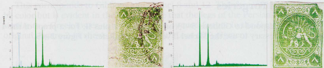
Figure 2-33. Additionally with a higher proportion of Lead (Pb) and presence of Chromium (Cr).
